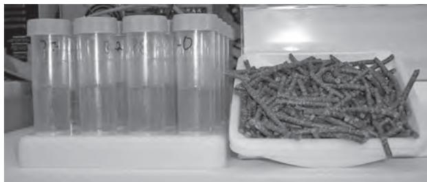
Canola oil and meal after seed crushing. After being weighed, the samples are analyzed for oil composition and quality.
