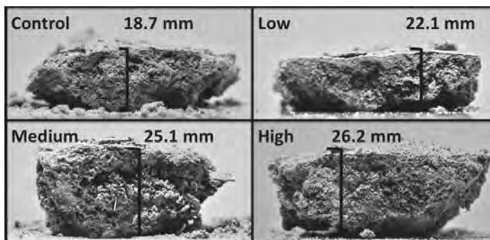
Fig. 1. Visual representation of crust thickness for each treatment.
